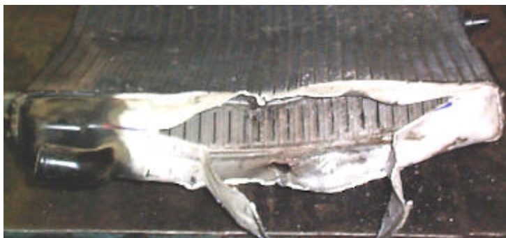
Motorcycle radiator damage before repair
