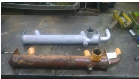
Tube and Bundle Marine Cooler Heavy duty replacement(right)
