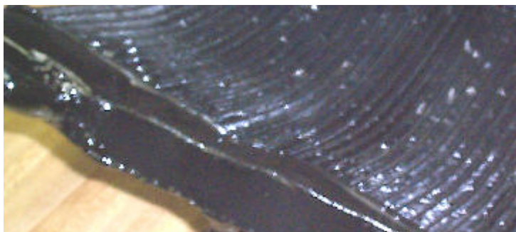
Motorcycle radiator after repair
