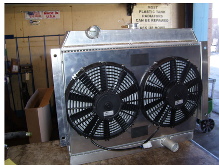
Custom Aluminum with extruded tube core, shroud and fans, '59 Cadillac 454
