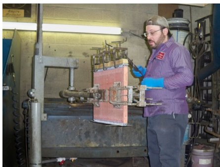
Repairing top tank on copper brass recore
