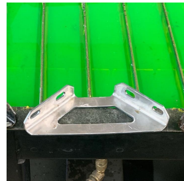
Designed Corner Brace for 3516 Caterpillar
