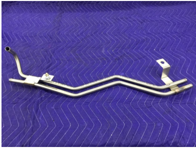
Stainless Steel School Bus Coolant Lines
