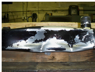
Repaired custom aluminum radiator. Bottom tank was damaged when a jackstand failed.
