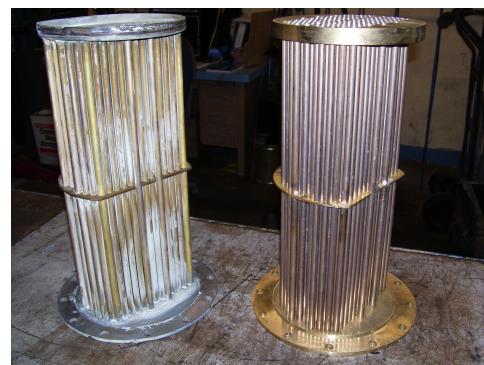
Tube and Bundle Marine Cooler Note, heavy duty replacement on right.
