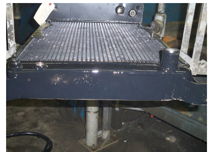
Repaired custom aluminum radiator. Bottom tank was damaged when a jackstand failed.
